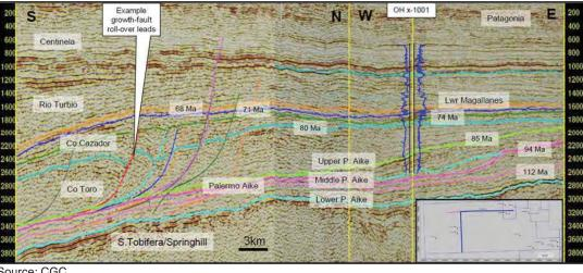
Figure 10: Seismic Section through the Tapi Aike Block showing Growth Faults in the CTC Section
